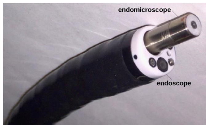
Fig. 9. Dual axes confocal endomicroscope can be passed through the 6 mm diameter biopsy channel of a medical endoscope (Olympus GIF XTQ180).
