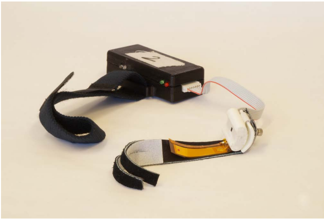
Fig. 1. The wireless version of the ring and the acquisition armband.
