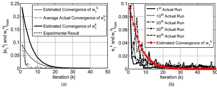
Fig. 3. (a) Average versus estimated convergence rate for the adaptive controller with SPSA (red lines) and experimental versus estimated convergence rate for the adaptive controller (blue lines). (b) Several single runs of actual convergence rate for the adaptive controller with SPSA.
