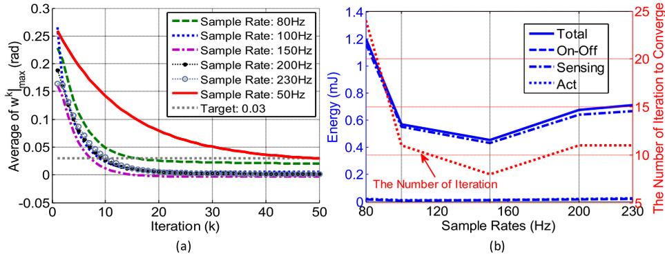
Fig. 2. (a) Estimated convergence rate with respect to sample rate, the changeable control setting for the heuristic search adaptive controllers. (b) Energy dissipation to reach the target error with respect to sample rates (Act: actuator energy. ON-OFF: switching drive circuit energy. Sensing: sensor circuit energy. Total: total energy for actuation, drive circuit, and sensing).
