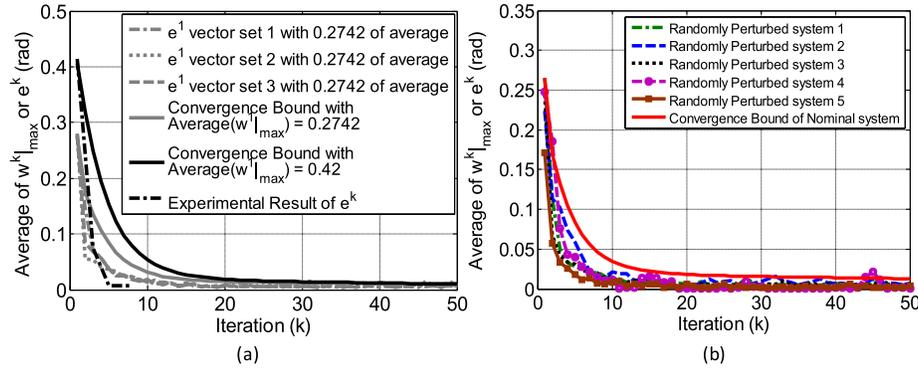
Fig. 1. (a) Convergence rate of several mean initial errors of output for the adaptive controller with heuristic search (red lines), and experimental versus estimated convergence (blue lines). (b) Several perturbed systems of actual convergence rate for the adaptive controller with heuristic search.
