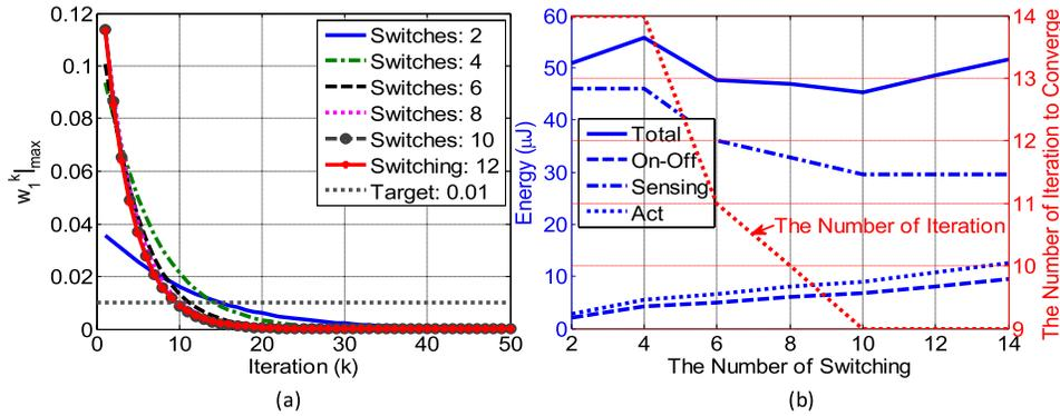
Fig. 4. (a) Estimated convergence rate with respect to the number of switching instance, the changeable control setting for the adaptive controller with SPSA. (b) Energy dissipation to reach the target error with respect to the number of switches per iteration (Act: actuator energy, ON-OFF: switching drive circuit energy, Sensing: sensor circuit energy, Total: total energy for actuation, drive circuit, and sensing).
